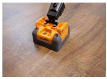
presence within its depth through conductance measurement. Another way, pinless meters tell you if there's moisture around, but not how much. For wood testing, this lack of specificity is helpful when trying to determine areas that require further investigation.
