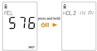
A scrolling text appears mentioning "hold in air and press right" hold the unit in air, away from any other object and then press key to calibrate the device for REL mode.
