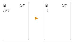
For example, if the Auto Off time is set as 1, then the unit will automatically shut down after a minute when no key is pressed.
